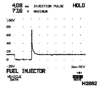
This multi-point fuel injection system is a conventional fuel injection system with a cut-off control system. In this case, the signal plot only has one voltage spike.
