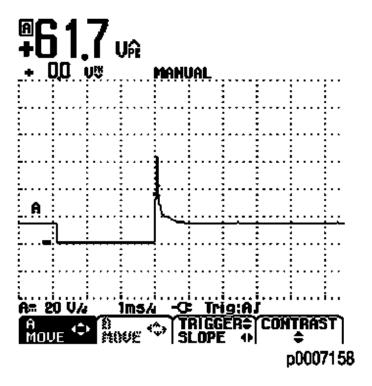
This multi-point fuel injection system is a conventional fuel injection system with a cut-off control system. In this case, the signal plot only has one voltage spike.
